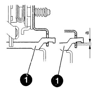
Adjusting control relay and starting-motor solenoid
